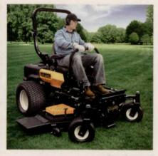
with a 37HP V-Twin air-cooled Kawasaki engine. Cub Cadet has also made improvements to its exclusive Command Cut System for improved durability, reduced maintenance and cleaner overall cut.
