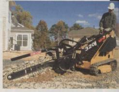
pressure to reduce damage to lawns and landscapes. The Boxer 320 is only 34.5 in. wide, but features a tip capacity of 1,250 lbs. and an operating capacity of 625 lbs. at 50% operating capacity. The 320 also has a ground speed of 3.4 mph and handles the same standard attachments as other Boxers. For more information contact Compact Power at 800/476-9673 or www.boxerequipment.com / circle no. 281
