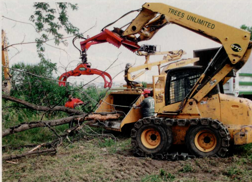
▲ A grapple attachment helps turn trees into mulch.
