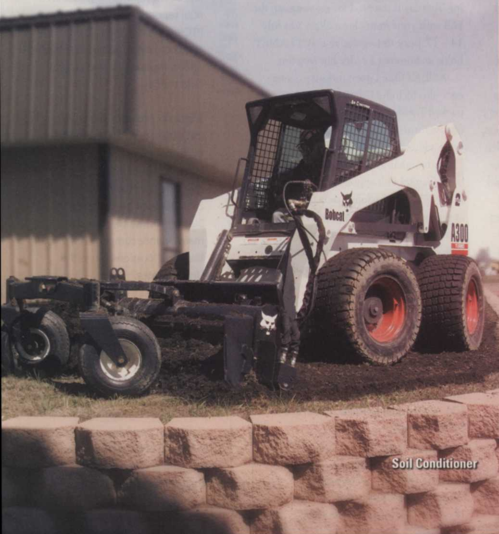
Rakes and collects surface debris.
