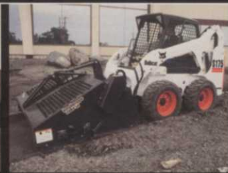
Skid-steer loader with Bobcat landscape rake.
