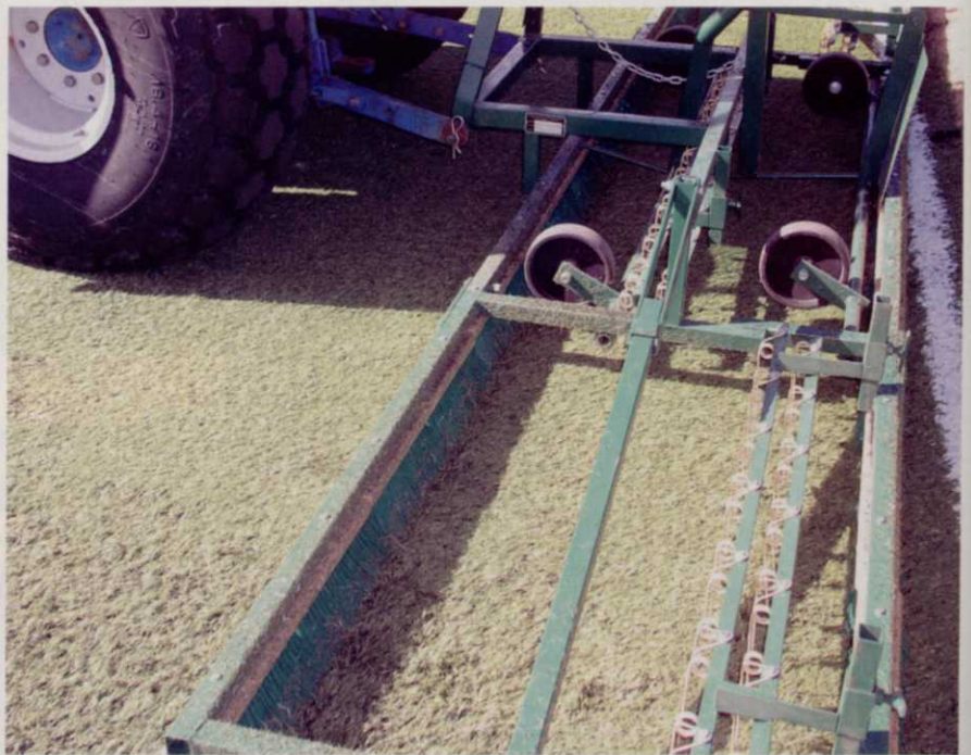
A rubber-infill artificial surface may require an athletic turf manager to drag it with a brush attachment that also has a scarifying unit to ensure the field doesn't get too hard.
