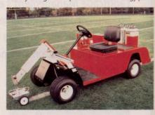
vides straight lines. Two 12-gal. steel tanks are controlled by a switch near the seat. A hydraulic spray arm sprays sharp, straight lines in front, or can be moved to the side for crisp circles.
