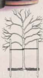
Typical ArborTie staking installation
