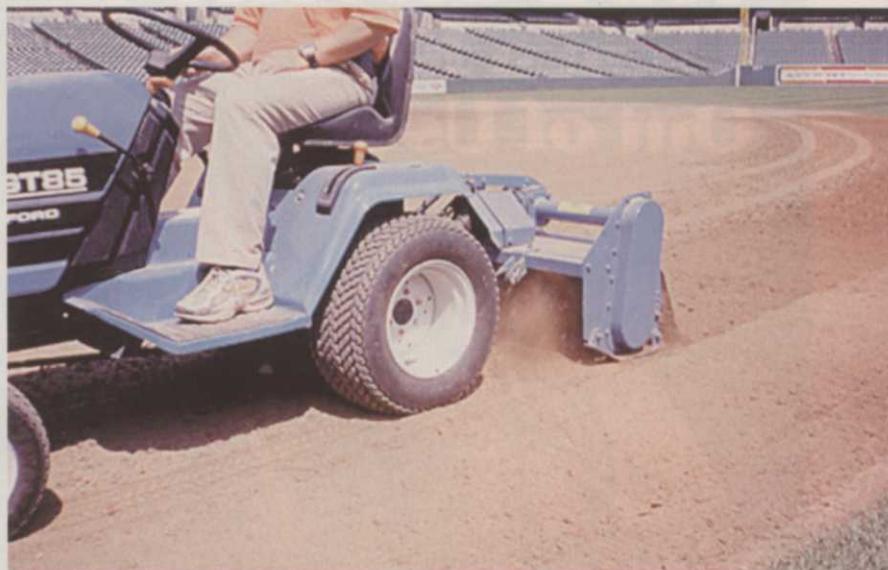
Rototilling calcined or vitrified clay products into an infield soil with too much clay or hardness will help fractionate it and make it more manageable.
