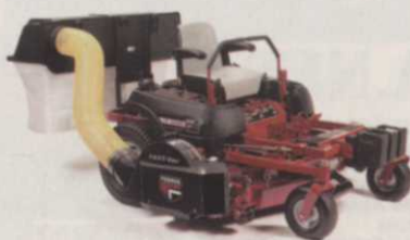
Fast-Vac System. Mows and vacuums in one quick pass. Unique side-panel air injection design handles more leaves and grass without clogging.
