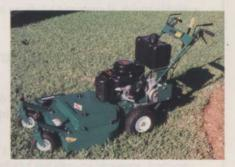
Mid-sized might Sarlo Power Mowers' Viper is a mid-size lawn mower, a five-speed and self-propelled machine with a 32-in.-wide cutting swath. Available with either a 10.5-hp Briggs & Stratton industrial-commercial, 12.5-hp Kawasaki, or 13-hp Honda engine. For more information contact Sarlo at 800/749-5296 or www.sarlomower.com / circle no. 258
