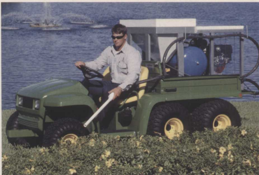
Cutler-Malone units with air-powered delivery via hand-held spray wand
