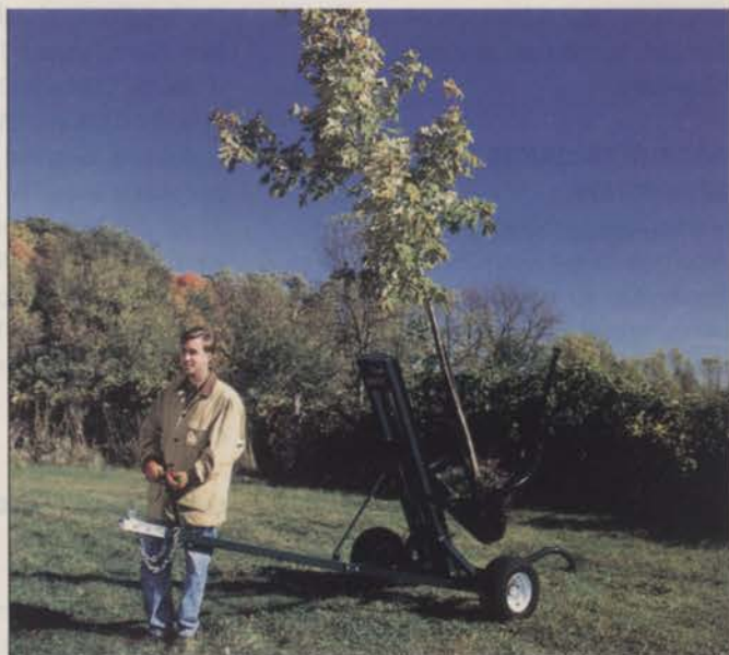
▲ Tree Toad can move trees up to 3 in. in diameter
