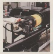
engine are accessed from curbside of truck. Powered by Kawasaki 5.5-hp FE-series engine and Hypro 403 series 3-piston diaphragm pump. Hannay electric hose reel has 300 ft. of 1/2-in. 800 psi urethane inner core hose. **Circle 268**
