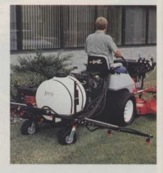
Plus engine with Udor diaphragm pump. The 3section breakaway boom has 5-, 8- and 11-foot spray patterns with zone control valves and ultra low drift nozzles. Gun with 10-ft. hose is included. **Circle 266**
