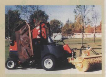
rpm. The broom has a sweeping path of 52 in. when angled 30 degrees left or right, while the rotary brush heads measure 25 in. in diameter and vary in lengths up to 60 in. Wire, polypropylene or 50-50 wire-polypropylene broom head options are available.
