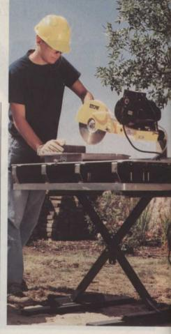
Stow Manufacturing says its TP-10 tile/paver saw is capable of ripping a 24-in. tile in a single pass or cutting an 18-in. tile diagonally. Powered by a totally enclosed, non-vented 1.5-hp electric motor, its blades range from 7 to 10 in. A 10-in. blade is standard, and additional blades and profiling wheels are also available. For more information contact BOMAG Light Equipment Division at 800/235-0008 or <a href="https://www.stowmfg.com">www.stowmfg.com</a> or circle no. 280
