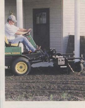
▲ The new Harley Power Box Rake for front-deck mowers can handle turf renovation and overseeding, dethatching existing turf or removing old or worn turf for reseeding. It operates driving forward, can windrow and grade to the right or left and can trap and remove unwanted debris with box endplates. It's available in 4- and 5-ft. models and comes with an adapter kit to fit most 22-hp front-deck mowers. For more information contact Glenmac, Inc. at 800/437-9779 or www.glenmac.com or circle no. 269
