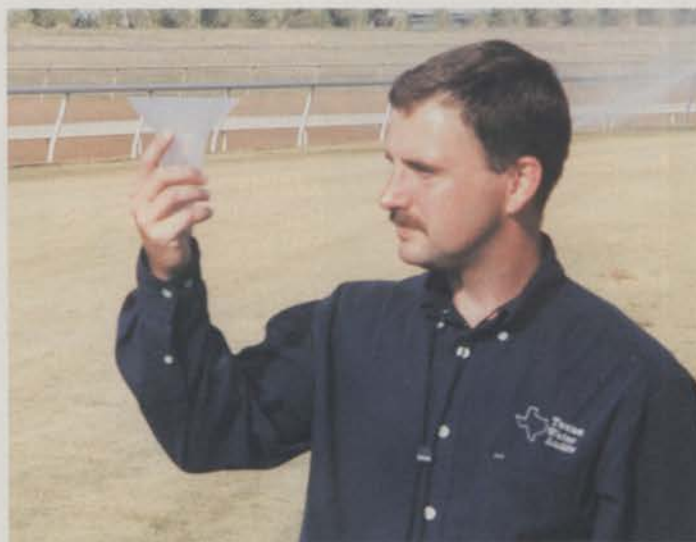
David Smith reads the volume from a catch device to determine sprinkler precipitation rate.
