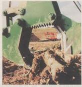
log shear attachment has a new universal mounting system that allows it to be adapted to any excavator. Adding the Megabyte now only requires that a bushing be inserted in the linkage arm. Made by Smoracy, LLC and marketed by Bandit, Remus, MI, it pulls
