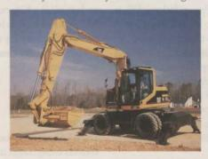
30,318 to 32,413 lbs. and is powered by a 113-hp Cat 3054 TA engine. The M315 weighs 35,082 to 36,228 lbs. and its 3054TA cranks out 114.2 hp.
