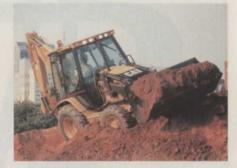
operated joystick controls. The 420D has 85 net hp and backhoe digging depth of 14 ft., 5 in. The 430D has 94 net hp and digging depth of 15 ft., 3 in. An extendable stick increases digging depths of 420D and 430D to 18 ft., 1 in. and 19 ft., 11 in., respectively. Both machines can handle applications involving pallet forks, material handling arms, brooms and buckets.
