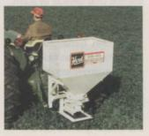
mount onto tractors with a Category I 3-pt. hitch, it's powered by the tractor PTO. It spreads fertilizer up to 36 ft. wide. **Circle no. 265**
