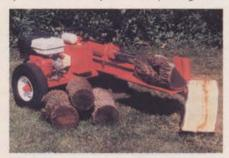
The tray has a 200-lb. capacity and holds logs up to 26 in. The Brute's splitting wedge design allows for more efficient log-shearing, even in knotty, twisted wood.
