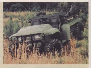
The cargo box has a 1,000-lb. capacity for a total payload of 1,400 lbs. The Gator can tow an additional 1,400 lbs.
