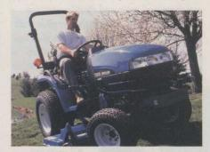
gear. For infinitely variable speed without clutch or shift lever, a hydrostatic transmission is available. Units have a 540-rpm rear PTO and a live 2000-rpm mid-PTO on models with hydrostatic transmission.
