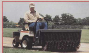
PTO-driven 48- and 60-inch fixed angle rotary brooms handle dirt, debris and clean up to eight inches of snow. 60-inch bidirectional broom available.
