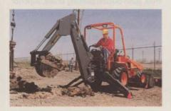
two-speed hydrostatic four-wheel drive and a weight of 4,570 lbs. Featuring a hydraulic PTO, it can power augers, tampers, breakers, drills and saws.
