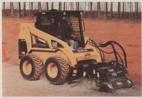
loaders feature high hydraulic horsepower to handle tools such as cold planers and stump grinders. The 228's and 248's operating capacities are 1,500 lbs. and 2,000 lbs., respectively. Each model has a Cat 3034 direct-injection, 4-cyl. diesel engine. Other features include pilot-operated joystick controls, more than 30 types of Cat work tools, and hydrostatic transmission that optimizes the hydraulic/rimpull match for greater productivity.
