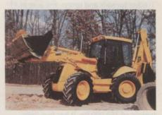
wheel drive, 4-wheel steer, four equal-size tires, 86 net hp JCB diesel turbo engine and SynchroShuttle transmission.
