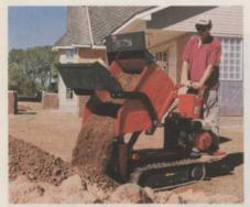
squeeze into hard-to-reach places. Its width can be reduced to 30 in., and ground pressure is dispersed evenly to minimize lawn damage.
