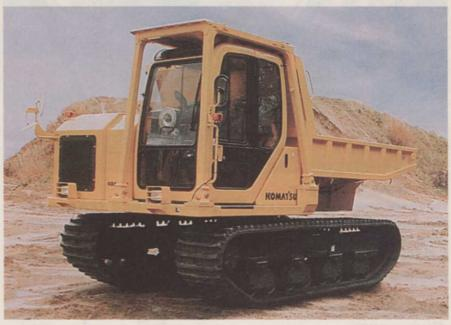
forward/reverse direction and the rotation of the upper structure. Driven by a 135-hp Komatsu engine, it has an operating capacity of 13,200 lbs., ground clearance of 19 in. and 3 psi ground pressure.
