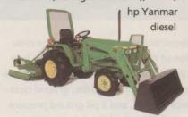
engine, PowrReverser™ transmission, four-wheel drive, independent PTO, lateral float rear hitch arms, planetary final drives), 790 (30-hp diesel engine, sliding gear transmission, optional four-wheel drive, optional selectable PTO), and 990 (40-hp Yanmar diesel engine, standard collar shift transmission, optional four-wheel drive, planetary final drive).
