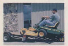
for side rails or provide convenient tie down points. A full axle and leafspring suspension make for smoother towing, molded fenders protect cargo from road debris, and built-in, anti-skid step pads in front and back allow convenient entry. Another feature is the rear gate/ramp that allows workers to drive an ATV, golf cart or riding lawnmower right onto the bed.
