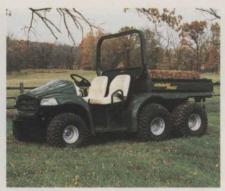
The vehicle also features variable speed transmission with rubber mounted engine and transmission, inboard wet brakes, differential lock and top speed of 19 mph. Load capacity is 1 400 lbs
