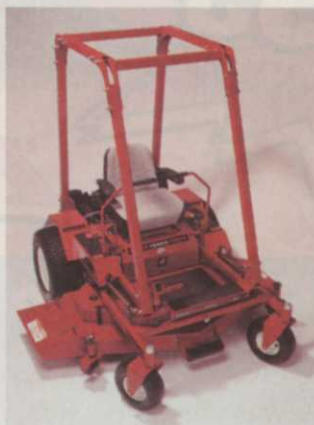
Ferris Industries' roll-over protection system
