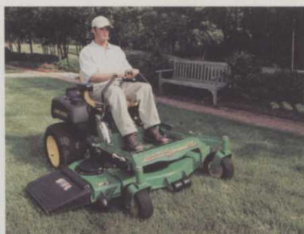
Deere M-Series mowers have antiscalp wheels
