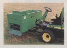
beds. It attaches to the John Deere 900 and 1100 series mowers and has a 3/4 cu. yd. capacity. The high-torque, 12-volt electric motor with switch allows the operator to regulate mulch flow from the tractor seat. Two agitators loosen the material as the mulch is discharged from the unit, then windrowed inside the edge of the bed.
