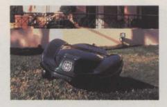
area to be cut, much like an invisible fence for pets. The mower moves in a random pattern, and changes directions if it hits a solid object. Husqvarna says it improves soil conditions since it cuts grass into tiny pieces that disintegrate. To deter theft, it is switched on with a personal code and has a built-in theft alarm.
