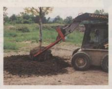
one to three trees to predug holes and releases, regrips, sets and holds the trees as one groundsman backfills to stabilize. Release to open the paddles, skid back and forth to backfill the hole, finish by hand and proceed to the next tree. "The Pincher" features same side load and unload from trucks and flatbeds. A hydraulic hose is included, but hydraulic quick couplers are not.
