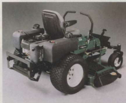
Lesco Viper features articulating front axle
