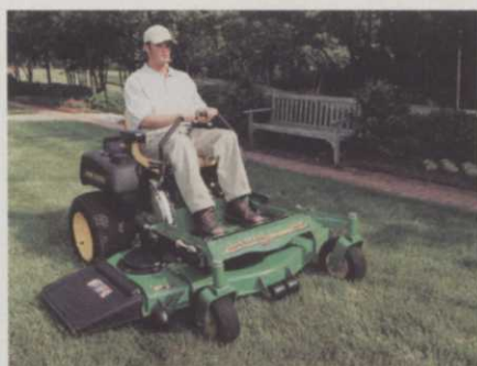
Deere M-Series mowers have antiscalp wheels
