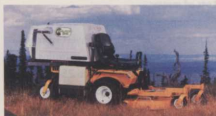
Walker MT with electronic fuel injection
