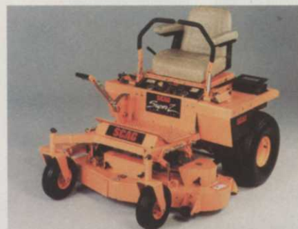
Scag Super Z with electric blade engagement
