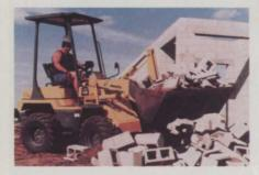
formance and skid steer versatility. A low effort single pedal allows for efficient control of speed and breaking. After dumping, the loaders feature a return-to-dig function that improves cycle times. The operator's compartment has dual
