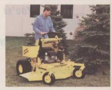
change. The Super Surfer is available in 36-, 48-, 52- and 61-in. cutter decks and engine options up to 23 hp.
