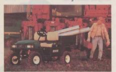
E-Z-GO Textron's new workhorse ST 480 features an 800-lb. payload capacity, 48-in. load bed and a 16-hp., 4-cycle 480-cc twin cylinder Vanguard V-twin engine, allowing the vehicle
