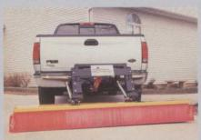
The snowman "multi-hookup" works all year. The 7 ½-ft. Grotech Broomer is available as a complete unit or as an attachment to Snowman plows. A straight or angle broom system is available. Easy installation of the complete unit is complete in under three hours.
