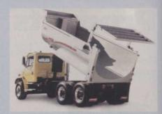
inch longsills also add to the low profile, while the absence of crossmembers prevents the washboarding that contributes to rust and corrosion. The new design, combined with the high-strength materials, is also more resistant to dents, and provides a faster, cleaner load dump.
