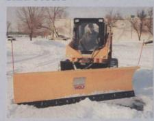
Snow Wolf is a snow plow designed for skid steer machines, with blade features and frame construction that maximize the greater snow-pushing strength of a skid steer, says the company.
