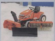
Kubota's G-Series garden tractors are equipped with standard two-wheel steering or optional four-wheel steering, ideal for confined areas.
