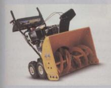
The Cub Cadet 4x4 Snow Thrower combines the technology of 4-wheel drive with a Regency OHV engine. The Cub Cadet 4x4 also includes fingertip-controlled power steering, heated handgrips and single-handed operation that frees the left hand to operate the 4v4's electric chute rotation.
