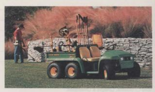
Gator is ideal for work areas such as college campuses and resorts. The unit's UL-approved charger plugs into a 120 VAC, 60-hertz wall receptacle and draws the maximum amount of current allowed to reduce charging time. Top vehicle speed is 15.5 mph. For more information, contact John Deere at 800/537-8233 or
