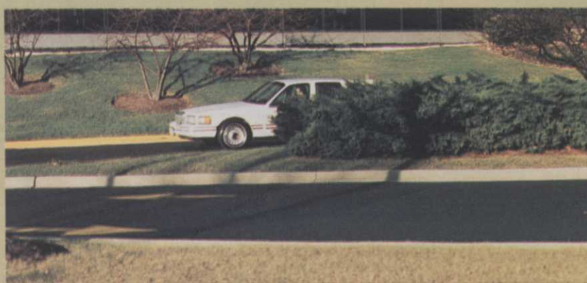
These overgrown junipers obstruct visibility and are dangerous. Lower shrubs would be safer and would be just as attractive in this location.
