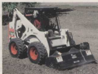
Tiller breaks up clumps, mixes material into soil.
