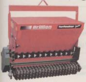
Due to the seeder's compact size, the Brillion Turfmaker Junior seeder, available in 4- and 6-ft. seeding width models, offers increased landscaping maneuverability. The 4-ft. model has a 7-bushel hopper capacity and 11 seed metering cups to evenly distribute grass seed, while the 6-ft. model can hold 11 bushels with 17 seeding cups.
