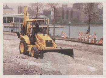
hp engine, compared to the 80-hp 555E engine. The LB75 is only available with 24-in. tires, instead of the 28-in. 555E tires
