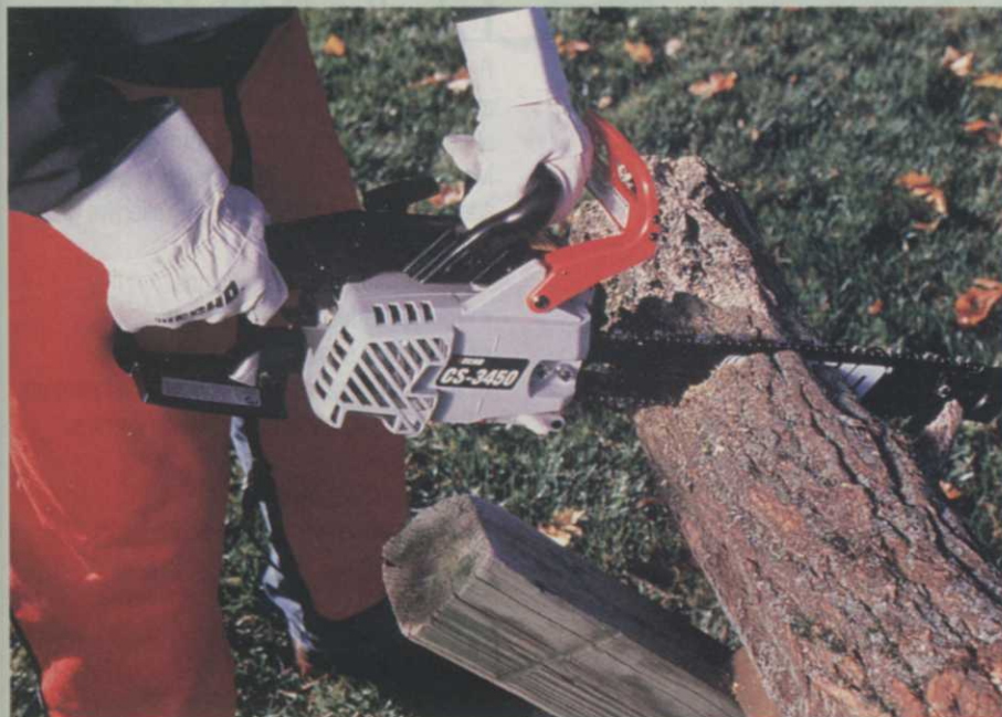
The Echo CS-3450 is available with a standard 16-in. bar and chain, but can be fitted with a 12- or 14-in. setup also. This model features the Slope Advance Ignition System.
