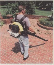
with a soft-tone muffler system, a pistol throttle and a 54-oz. fuel tank. Operating at 7,000 rpm, the blower has a 69.5 dBA rating at 50 feet.
