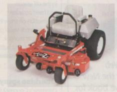
tive than ever. The mower has either a 20-hp or 23-hp Kohler Command Pro engine or the 23-hp Kawasaki engine. The Exmark has ground speeds of up to 9.5 mph forward and 4 mph in reverse.
