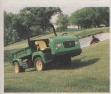
versions, features a five-speed, synchronized transmission and a one-piece axle for rear-wheel support. The vehicle also features front and rear dual spring leaf suspension, a turning radius of 33 in. and a 2,650-lb. load capacity.
