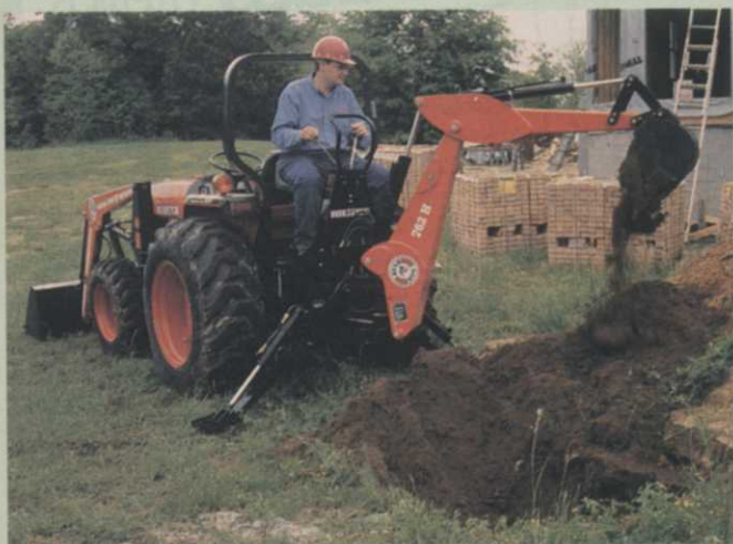
Bush Hog 762H accepts either regular or heavy-duty buckets in 9-, 13-, 16-, 24- and 36-in. widths. Maximum reach is 9'6".
