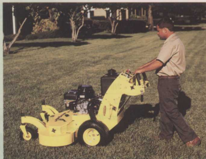
Great Dane Scamper offers 36-, 48-, 52- and 61-inch cutter decks.
