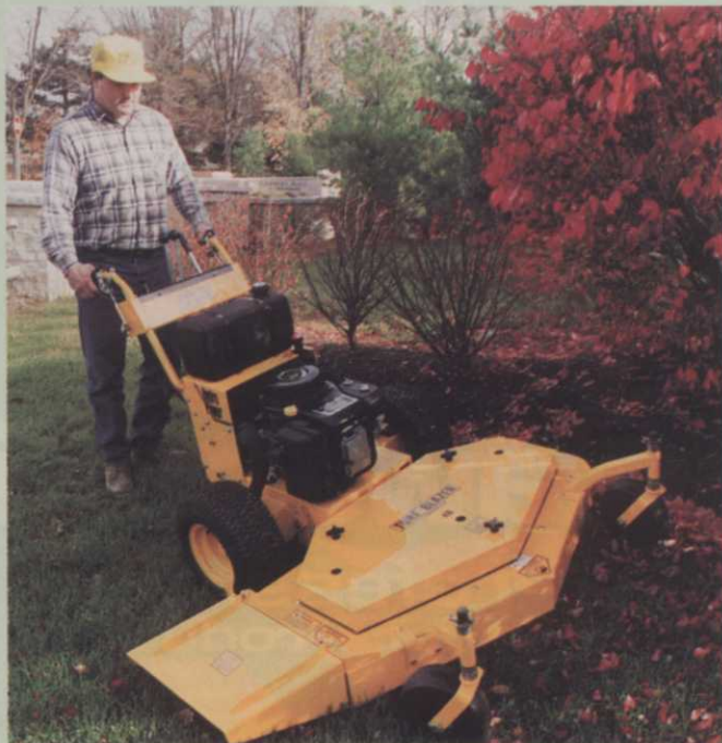
Howard Price Hydro Walk-Behind features dual hydro control levers. Floating deck system oscillates to prevent scalping.
