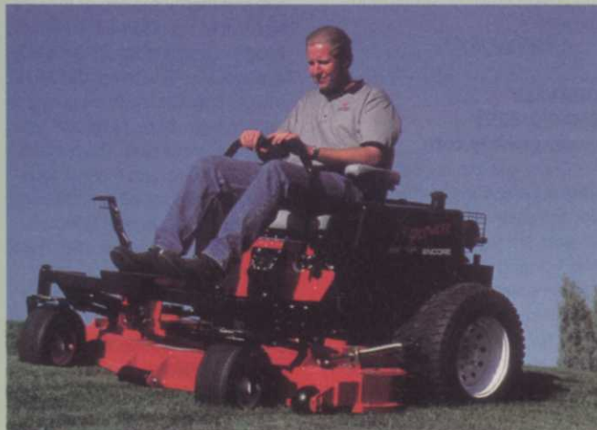
Encore's new 61-in. Powler Mid Cut is powered by a 22-hp, liquid-cooled Kawasaki. The unit rides on 24-in. Super Turf tires.
