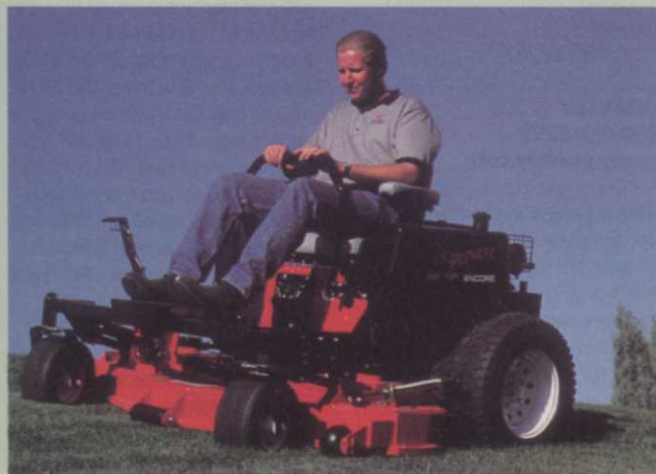
Encore's new 61-in. Powler Mid Cut is powered by a 22-hp, liquid-cooled Kawasaki. The unit rides on 24-in. Super Turf tires.
