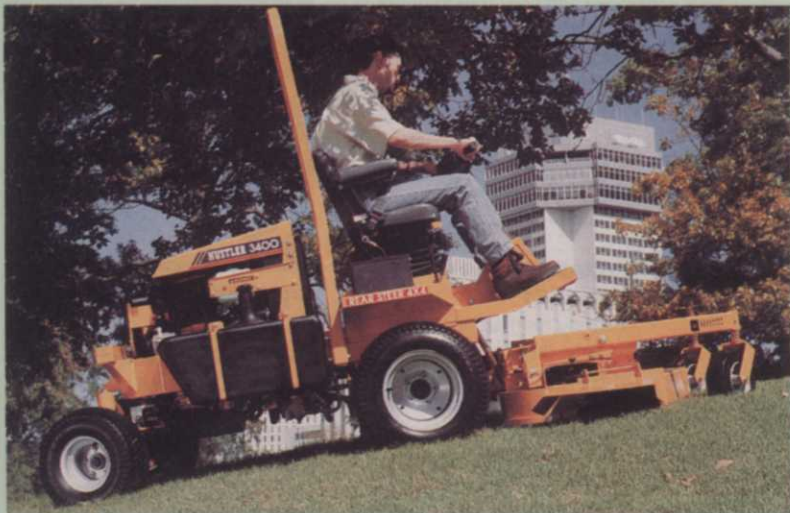
Excel Industries continues to offer unmatched traction and stability with its new all-wheel-drive 3400. Hustler uses the easy-to-use H-bar steering system.
