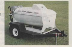
mount on a flatbed truck along with an auxiliary water tank or will fit into the back of a pickup. It is also available mounted on a trailer with a 5,000-lb. axle, electric brakes and heavy duty tires. The unit can be removed from the trailer if desired.
