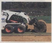
wide sod rolls. The Sod Layer speeds sod laying 2 to 3 times over that of hand labor but is less expensive than a dedicated sod-laying machine. The attachment has a cutting blade, auxiliary hydraulic controls and relief valves.
