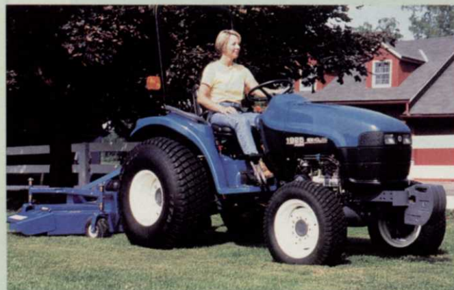
Model 1925 Boomer tractor powered by 34-hp diesel from New Holland. "Boomers" also available in 25, 27 and 29 engine hp.
