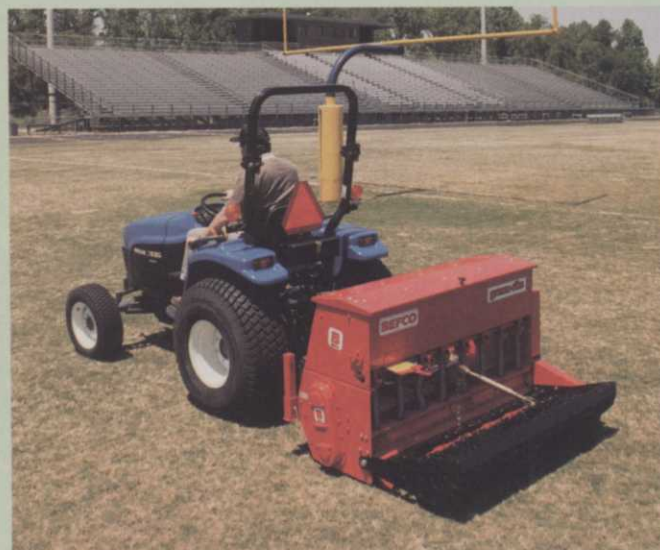
Befco's Green-Rite aerator/overseeder aerates, seeds, agitates seed to the ground and compacts the seed in a single pass.
