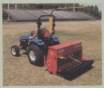
Befco's Green-Rite aerator/overseeder aerates, seeds, agitates seed to the ground and compacts the seed in a single pass.
