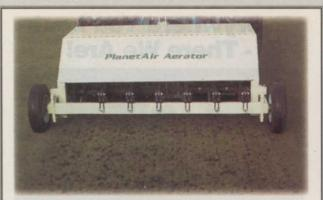
The *Planet Air* aerator, with its patented planetary motion and unique coring tine design, relieves the hard pan effect. The 12 tines penetrate the earth to depth of 4 inches with a span of 48 inches wide. The tractor's forward speed determines hole spacing, making the *Planet Air* highly productive with low PTO horsepower requirement. Clean up is minimal due to its pulverizing capability.
