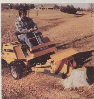
faster than a self-propelled, trailer or walk-behind type stump cutter. Hustler power plants come in 23, 28, 38 or 54 hp and the 15-in. diameter cutting wheel can cut stumps from 15 in. above ground to 10 in. below ground.
