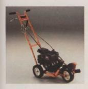
10-in. milled-edge blade for heavy duty edging and a longer life. Constructed of 0.25 by 0.25-in. bar stock, the edger has no movable parts near the drive head, no springs to break and no sliding boom or tilt quadrant to wear out. The blade head is a solid mounted boom, with belt-tensioning idler pulley and sealed ball bearings.
