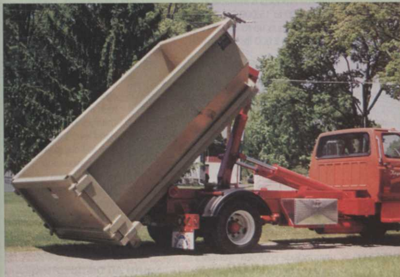
Hook-All Hooklift trucks from Automated Waste Equipment have a single rotation point and dual-lift cylinders rated at 2400 psi hydraulics.
