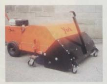
using only two quick pins and a lever, makes for easy dumping of the 2.5-cu. ft. hopper. The floating design allows it to stay right in the path of the debris coming off the broom and keeps the hopper from interfering with the broom as it moves across uneven surfaces.
