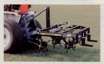
52 core plug aerator allows the operator to aerate while turning in any direction, no matter how sharp the turns.
