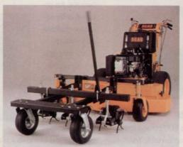
ing mowers. The 38" wide aerator has zero-turn maneuverability with up to a 3" hole depth and can aerate 66,000 ft<sup>2</sup> per hour at 5 mph.
