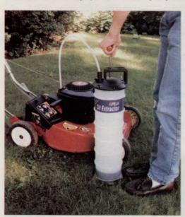
from the engine crankcase. The integrated container holds 1.7 gallons, preventing spills and has a built-in float switch which automatically shuts the pump off once the container is full. This tool eliminates the need to remove drain plugs when changing oil. The Oil Extractor is
