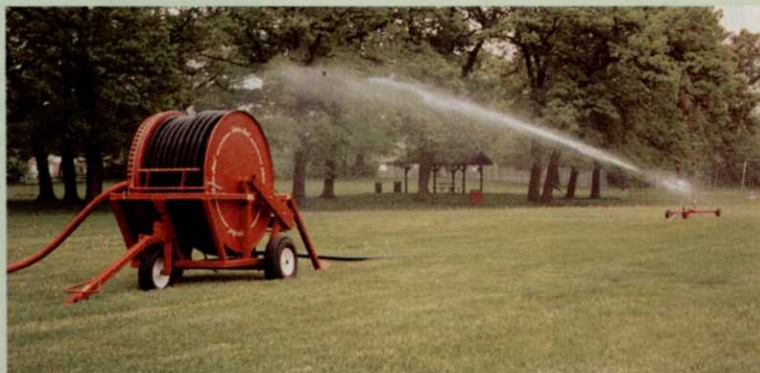
Kifco, Inc.'s B140 can irrigate a football field (about one acre) in a single pass.
