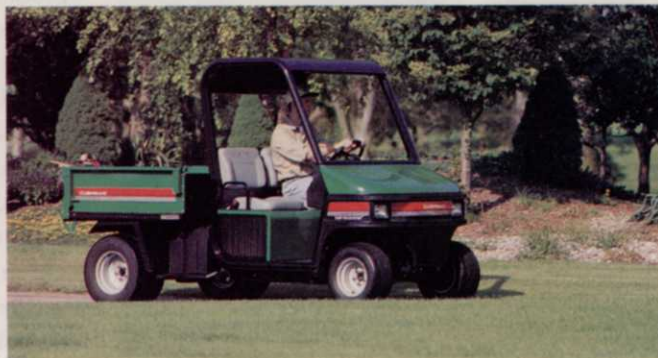
4-wheel Turf-Truckster rated at 2,600 lbs.
